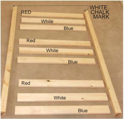
First we need to create headboards. The corner posts have a white chalk marking. VERY IMPORTANT - these indicate the top of the post, at the base they will have PNL - (left side) and PNR - (right side). Select one of each, place 1x PNL to the left, PNR to the right.
