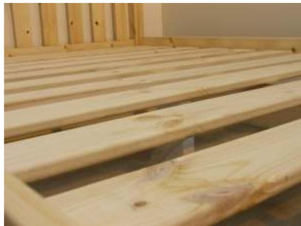
Now push the slats flush to the left hand side rail and screw in (do not screw the right hand side yet). Now go to the right hand side and start with the slat near the centre. Push the side rail in so the slat is flush, then fix using the screw. This aligns the side rail. Now fix the remaining base slats.
