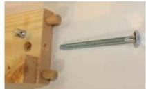
Firstly ensure there is no sawdust or debris in the access holes. Using a bolt push through to clear. Now insert the dowel rods at all ends, do not push all the way in.
