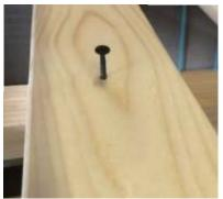
TIP:-When you have attached the base slats you will have additional base slats screws. Out of the 12 slats screw 4 of them directly into the centre rail. Using the base slat screws simply drill through the top of the base slat into the centre rail. This will further strengthen the bed.
