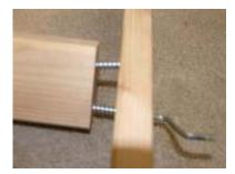
When installed the ladder rungs need to be tight. The holes on the ladder struts have been misdrilled by 2mm to ensure a tight fitting. Locate each ladder to the holes on the long struts. Using the small confirmat bolt dip them in the glue and push BOTH through the strut, you will note they will not quite meet the hole on the step.
