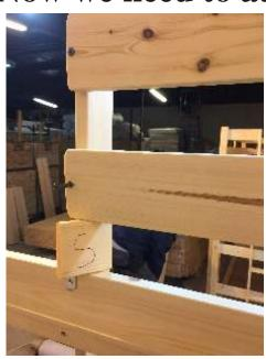
First select the bottom front guard rail (part 7) marked white. Using fixings A attach to the corner post. Rest the spacer bar (fixing A2) as shown in the picture at the end of the rail. This will ensure the correct gap is allowed.
