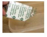
Open the sachet and empty into a plastic container. Whenever you connect a confirmat bolt (D) or a connector bolt (B) into a barrel bolt (c) dip the end of the bolt in the wood glue and screw in as normal. This will act as a lock tight and prevent the bolt from working loose.
