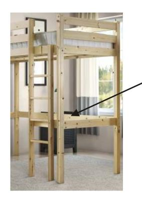
The bottom rear of the bed requires a Bottom rear brace (Part 17)to prevent the legs from moving apart. This part is coloured coded,
