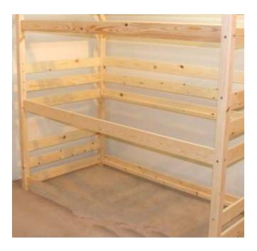
We now need to attach the two front side rails, the guard rails are attached later. again using fixings B and C attach as per the above picture. These are fixed to the third and sixth set of holes on each corner post. Once fixed you can now tighten all fixings ready for the next phase.
