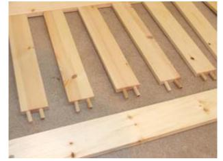
Lay two headboard facias marked Black PART 9 (4G) position these as shown in PIC 1. Lay the long inserts (PART 12) in between these ready to join.
