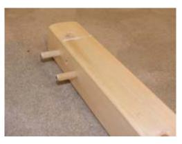
Now, remember to ensure the WHITE CHALK markings are facing upwards locate the dowel rods to each corner post. Again, do not push in the dowels all the way. Once in place connect the head board to the corner post, you will again see the dowels align as you tighten. Then fix using the bolts below.
