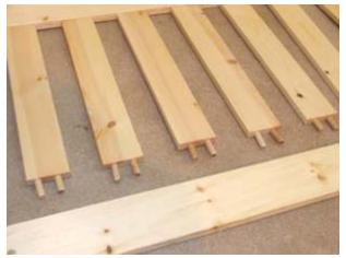
Place dowel rods in all the headboard LONG inserts as described, DO NOT PUSH ALL THE WAY IN. Now locate the PART 9 facias and push in to create the headboard. The dowels will straighten as they align.
