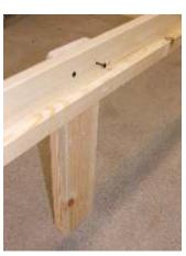
It is important this leg is attached as it supports the side rail. Measure a half way point on the side rail. Place the support leg under the side rail from the outside. Using two black screws attach from the inside of the side rail. Note there is no access hole as the screws are self threading
