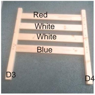
Now we need to build the right hand headboard (as standing in front of the bed). Locate the following parts and position as per the photo:
