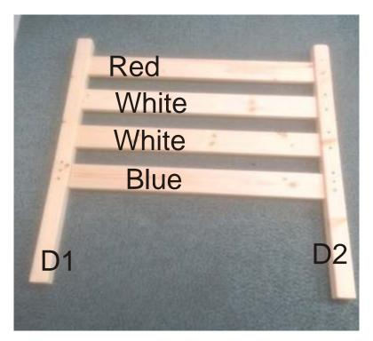
First we need to build the left hand headboard (as standing in front of the bed). Locate the following parts and position as per the photo:
