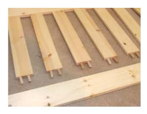
Place dowel rods in all the headboard inserts as described, DO NOT PUSH ALL THE WAY IN. Now locate the PART 9 facias and push in to create the headboard. The dowels will straighten as they align.
