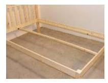
From the inside of the bed we need to attach metal brackets, one either end. These are fixed using the small screws (L), these are fixed to bottom headboard facia. Using a tape mark a centre line from each corner post, then measure and mark **55mm** from the top of the BLUE Facia(13). Now position the top of the bracket (J) just below this mark, attach with the small screw (L)
