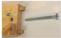
Firstly ensure there is no sawdust or debris in the access holes. Using a bolt push through to clear. Now insert the dowel rods at all ends, do not push all the way in.
