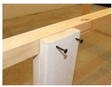
The centre leg is located under the centre rail, in the centre. Simply measure to the centre of the bed and locate under the centre rail. Using two black screws attach from the side.
