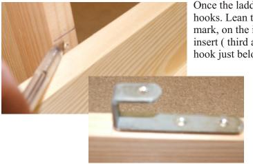
Once the ladder has been built we need to fix FOUR x ladder hooks. Lean the ladder against the end rail. With a pencil mark, on the inside mark the top of the each blue headboard insert (third and sixth one down). Now screw the ladder hook just below this mark and to the top of the smaller strut.
