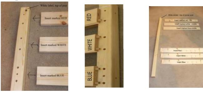
We need to build the two headboards at either end of the bunk bed. You will find four corner posts, On the BOTTOM of the post they will be marked with an end letter "L" and "R" (left and right)
