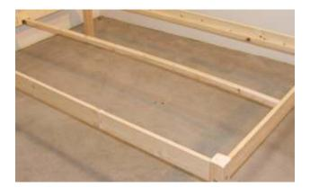
From the inside of the bed we need to attach metal brackets, one either end. These are fixed using the small screws (L), these are fixed to bottom headboard facia. Using a tape mark a centre line from each corner post, then measure and mark **55mm** from the top of the BLUE Facia(13). Now position the top of the bracket (J) just below this mark, attach with the small screw (L)
