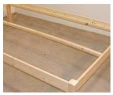
Firstly ensure there is no sawdust or debris in the access holes. Using a bolt push through to clear. Now insert the dowel rods at all ends, do not push all the way in.
