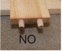
Now push the dowel rods in either side of these headboard facias. It is IMPORTANT, do not push these all the way in. Have them loose so they can angle when you attach. They will align when you attach to the post.
