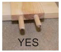
Now, remember to ensure the WHITE CHALK markings are facing upwards locate the dowel rods to each corner post. Again, do not push in the dowels all the way. Once in place connect the head board facias to the corner post, you will again see the dowels align as you tighten. Then fix using the bolts below.
