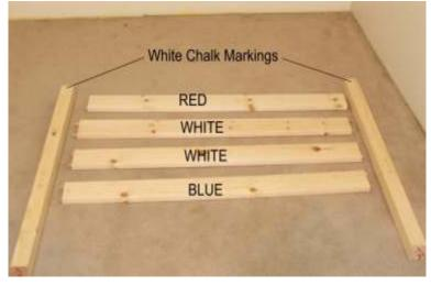
First Select the two headboard posts, See page 4 for corner post codes (post codes ending in L are Left side, ending in R are right side) Lay each post on the carpet, these posts will have a white chalk marking, these MUST be facing you and at the top when laying on the carpet.
