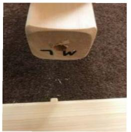
We now need to attach the bottom headboard facia 4E. You will note this has a dowel hole on the top, please locate a wooden dowel. This now connects to the bottom of corner post ML.
