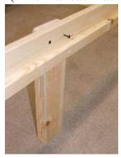
It is important this leg is attached as it supports the side rail. Measure a half way point on the side rail. Place the support leg under the side rail from the outside. Using two black screws attach from the inside of the side rail. Note there is no access hole as the screws are self threading
